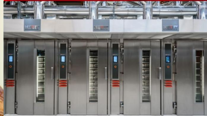
*Thanks to the excellent heat retention capacity of the transfer medium, short interruptions do not result in instant cooling and do not affect the quality of the end product. It comes as no surprise that bakers in small and large bakeries are full of praise for the VULKAN THERMO-ROLL oven, which is available in various sizes and models.*
